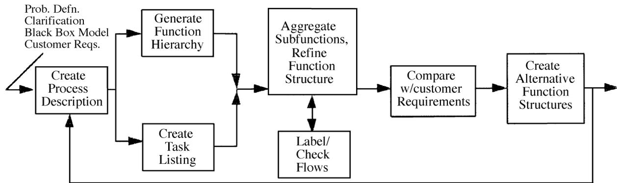
Fig. 3. Functional modeling and analysis process.
