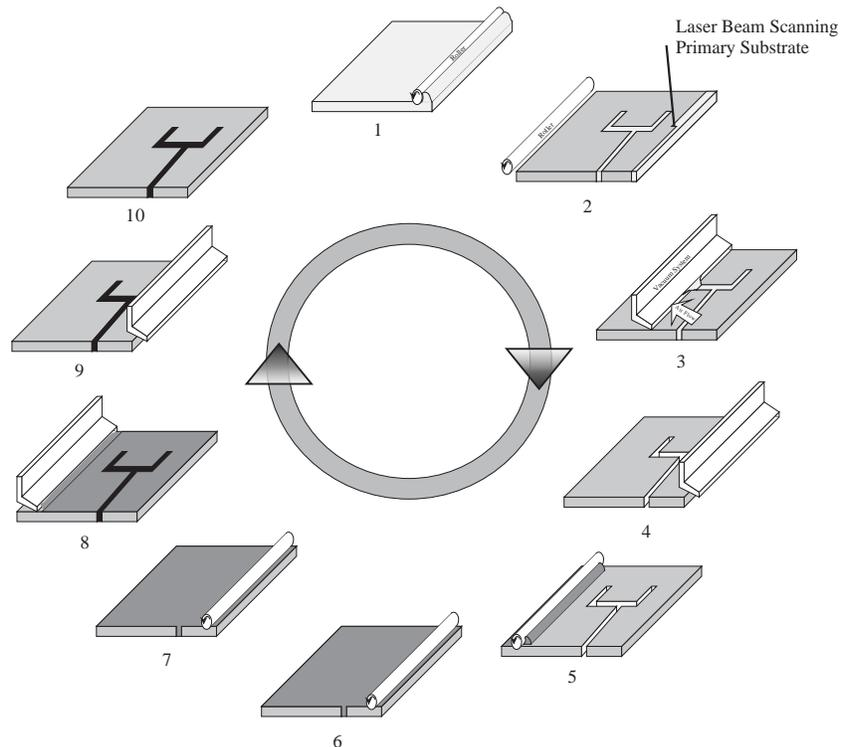
Figure 6. Conceptual design of multiple material SLS process.
