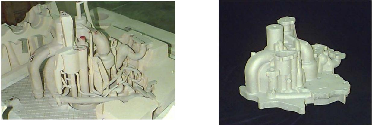
Figure 5. Core array and finished casting.
