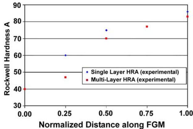
Figure 7. Correlations between FGM distance and hardness.
