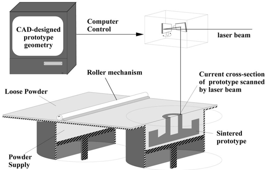
Figure 1. The selective laser sintering process.
