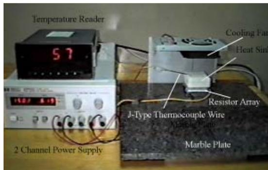
**Figure 15: Overview of CPU Cooling Experiment**
