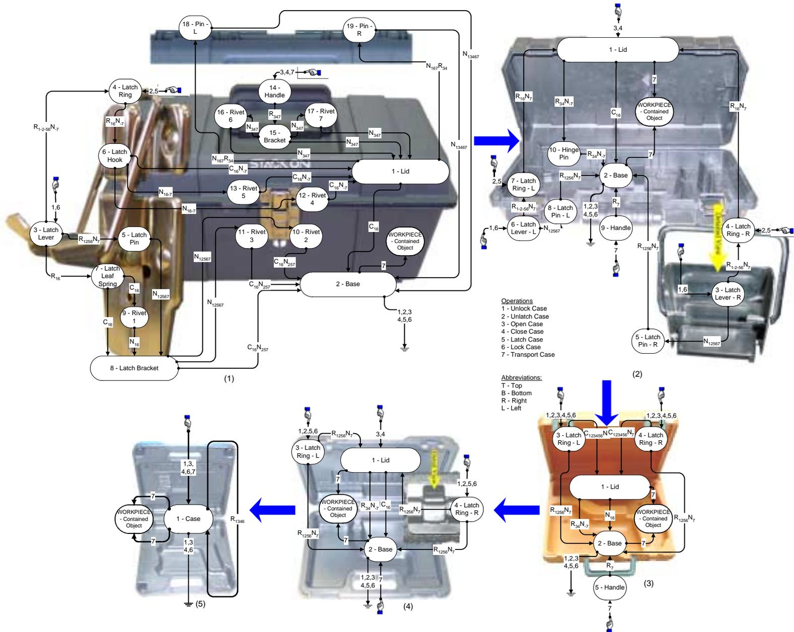
Figure 13: Effort Flow diagrams for Baseline and Evolved Tool Box Products.
