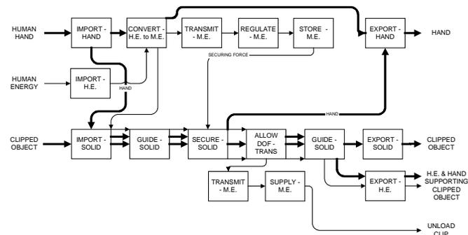
**Figure 6: Kitchen Clip Function Structure**
