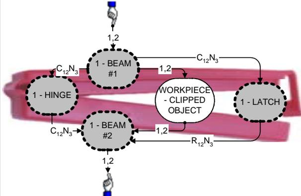
**Figure 10: Resulting monolithic structure shown as functional components in clip product**
