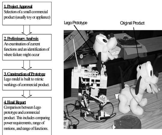
**Figure 3. Project Tasks in the Lego “Reverse Engineering” Project: Comparison of Walking Dog Prototype and its Commercial Counterpart**
