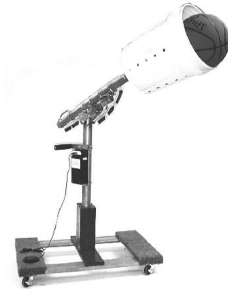
**Figure 9: Switch Activated Ball Thrower<sup>34</sup>.**
