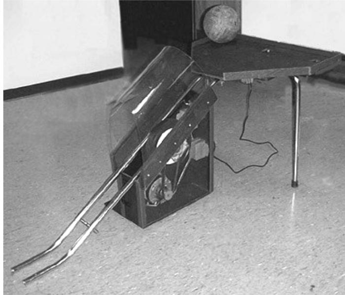
**Figure 7: Assistive Bowling Device<sup>35</sup>.**
