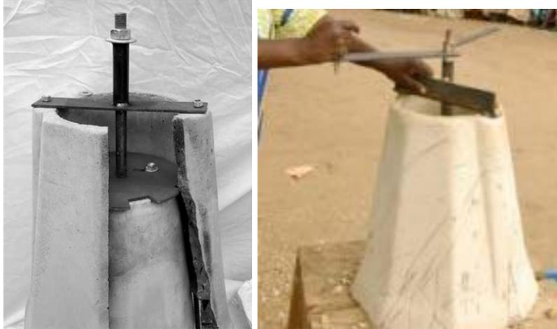
Figure 7: Participants in the control group only found within domain solutions to the peanut shelling problem. This solution is a hand-powered device that removes the shell from the peanuts (“Full Belly Project”, 2006).
