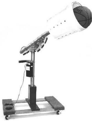
Fig. 5. Switch activated ball thrower [41].
