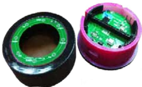
• **BWard Real-time Blood Sensing and Wound Monitoring Device**
