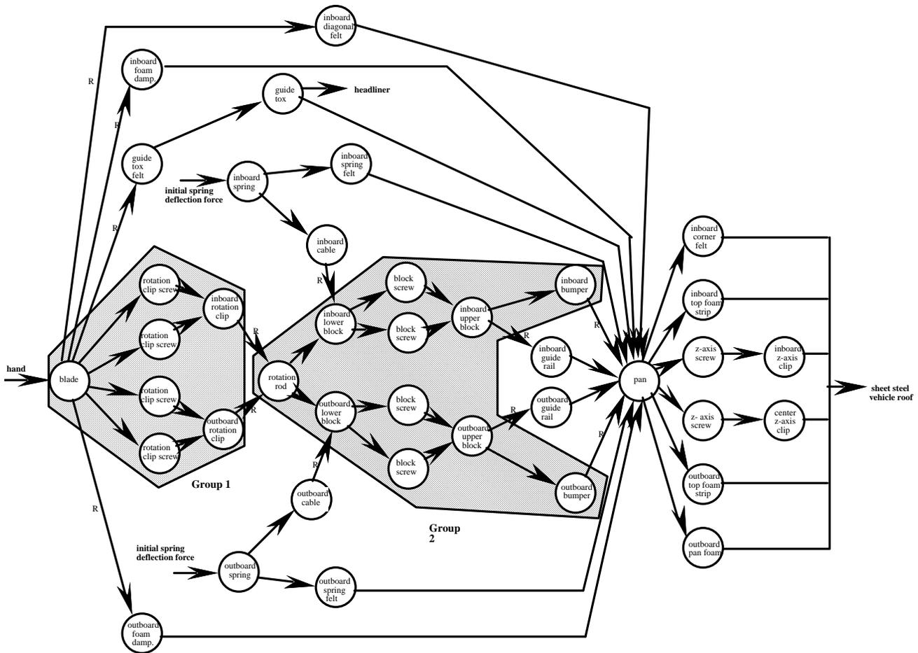
Figure 10. Force Flow Diagram of the SOAV.
