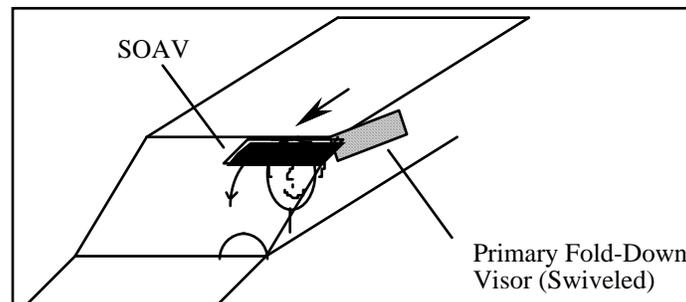
Figure 8. Simple Schematic of SOAV.
