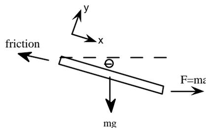
Figure 12: "FBD" of Linear Friction.
