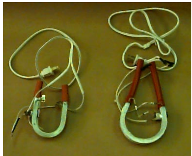
Fig. 6. The convert electricity to thermal energy module for the Brand A tea brewer (left) and the Brand A coffee maker (right).
