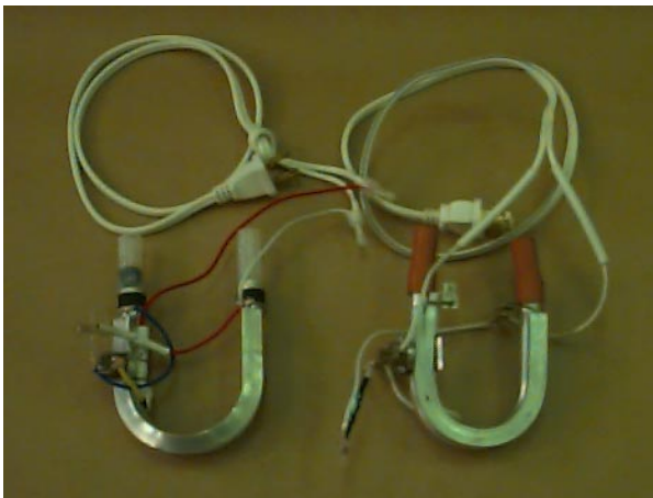
Fig. 3. The convert electricity to thermal energy module for both tea brewers.
