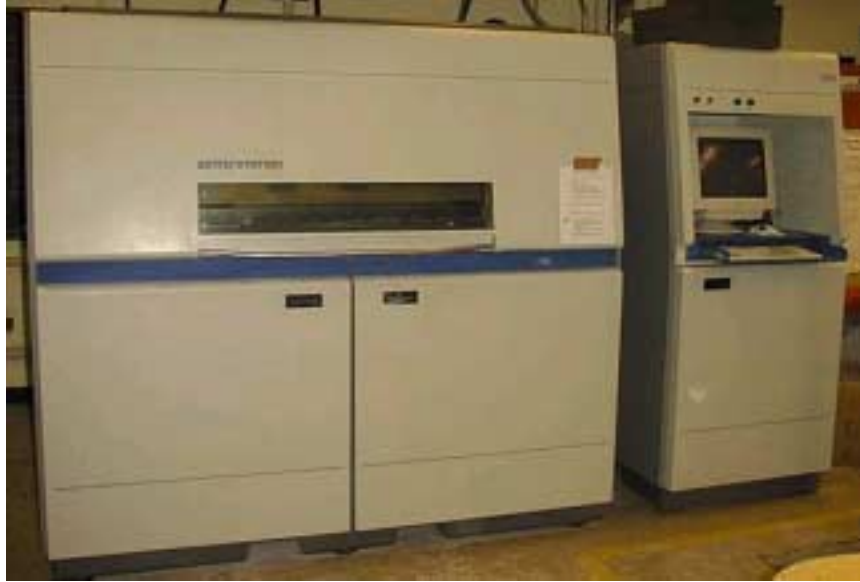
Figure 3: DTM Sinterstation 2000 in the UT SFF Manufacturing Laboratory.
