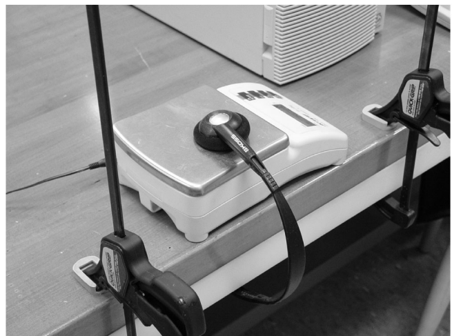
Plate 4 Experimental setup for headphone tests
