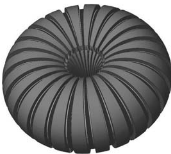
Figure 10 Toroidal fuel cell stack design
