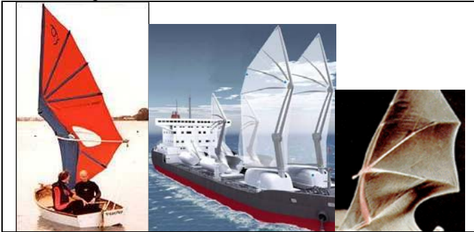
Figure 1: The sails of this cargo ship are designed based on an analogy to a bat's wing [4,5].
