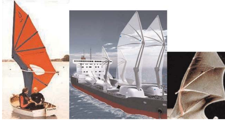
Fig. 1. The design of the sails of the cargo ship are based on analogies to a bat's wing (left panel, BBC, 2000; middle panel, Reed, 2006; right panel, adapted from Scientific American , 1998).
