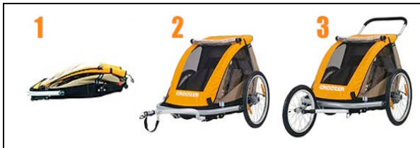
Figure 4. Three states of the Croozer 535 child carrier: (1) storage, (2) bicycle trailer, and (3) jogging stroller [31].
