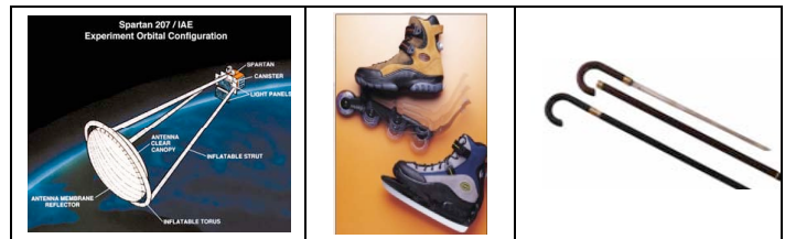
Figure 3. Examples of the three indicators: The IAE satellite deploys by inflating [21], inline and ice skate modules attach to a core boot structure [22], a cane conceals a blade [23].
