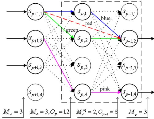
Fig. 2. Simplified QRDM trellis diagram ( $M = 4$ ).
