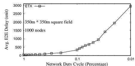
Fig. 1. E2E Delay vs. Network Duty Cycle
