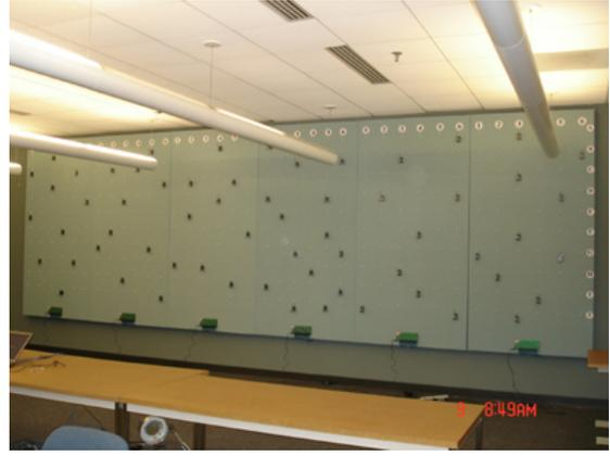
Fig. 2. the new developed Test-bed of Wireless Sensor Network
