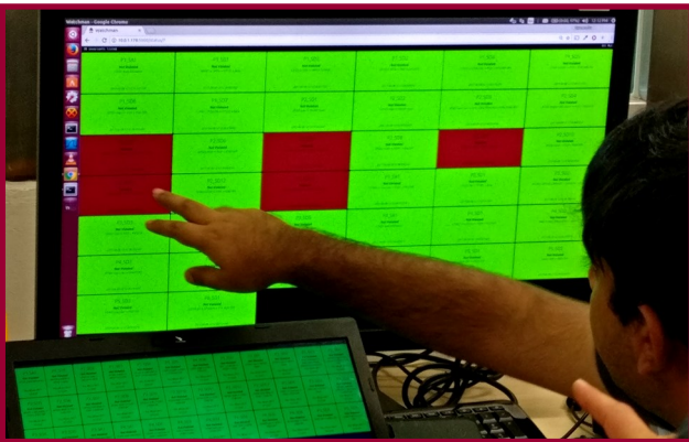
iTrust’s defence mechanism, the Water Defence Historian, detecting attacks (red boxes) as they occur
