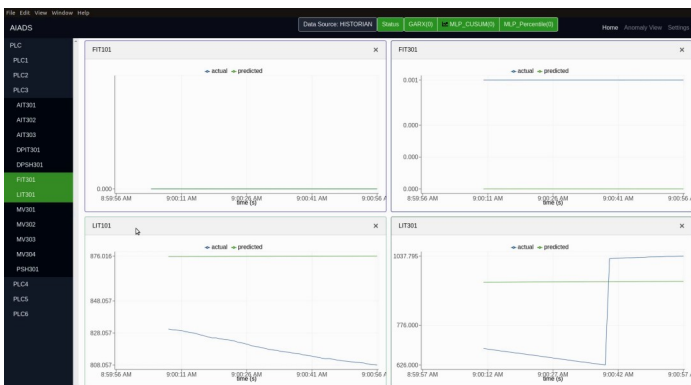
Fig. 8: Four subplots of PlantViz showing actual and predicted values in various stages of SWaT
