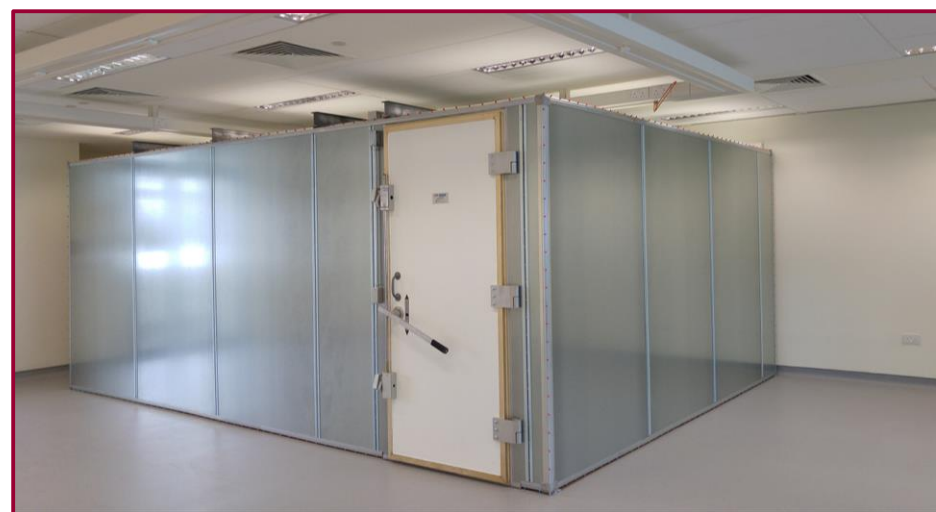
A Radio Frequency (RF) shielded room in the IoT laboratory
