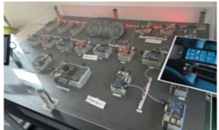
Fig 8.: Control system rig for exploring cyber attacks on autonomous vehicles
