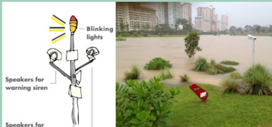
Diagram of a safety node (left), a safety marker with speaker (right)
