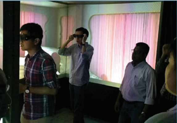
SUTD's own VR Cave' is a tri-projector setup developed by Aviation Virtual Pte Ltd, who also built Changi Airport Group's VR system for aerobridge training. The system allows users to view the front, left and right side of the environment with a pair of glasses. Each projector screen is about 2m by 2m, which allows users to be immersed in the environment itself. The glasses are equipped with sensors that can detect head movement and increases the visual accuracy relative to position of the users.
