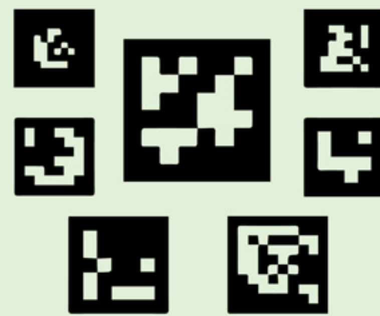
Markers Made Up From Black And White Grids Can Be Detected By Computer Vision
